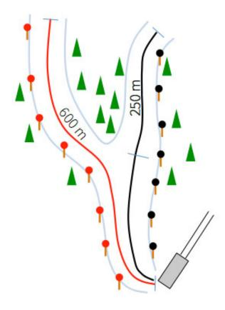
Measuring method Schrahe / FIANET / OITAF: single measurement of parallel segment = 850 m
