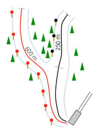
Measuring method Schrahe / FIANET / OITAF / WKO and Seilbahnen Schweiz: single measurement of parallel segment =  $850\ m$
