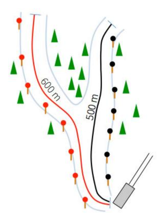
Measuring method WKO / SBS: double measurement of parallel segment = 1100 m
